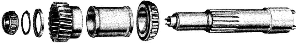
Fig.2 Servo driveshaft assembly dismantled
