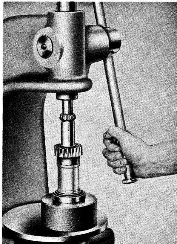
Fig. 3 Pressing bearings into position
