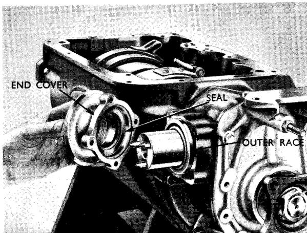
Fig. 1 Removing end cover
