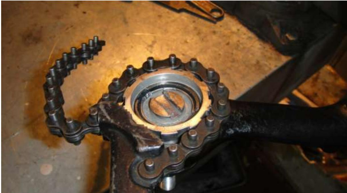
And here we have Madam Lash, as I like to call my chain wrench, entwined about the retaining collar securing the top ball joint bearing. Having removed the retaining ring above I realised that it was not really necessary unless you need to replace the bearing housing itself. Anyway it made cleaning the whole thing easier to clean and allowed fitting of a thick bastard in the slot of the adjusting cap.
