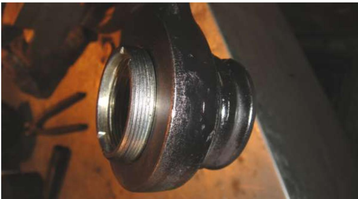
Retaining ring off, the rubber boot can be left in place if it's in good condition. Note the slots machined in the top of the bearing casing. The slots in the housing are provided to allow the adjusting cap lip to be peened at these points to lock it in place.
