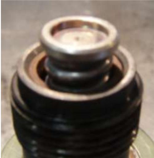
Here we have the other end of the switch with the brass terminal (7), its stepped insulator (8), the spring (5) and the contact disc (6)
