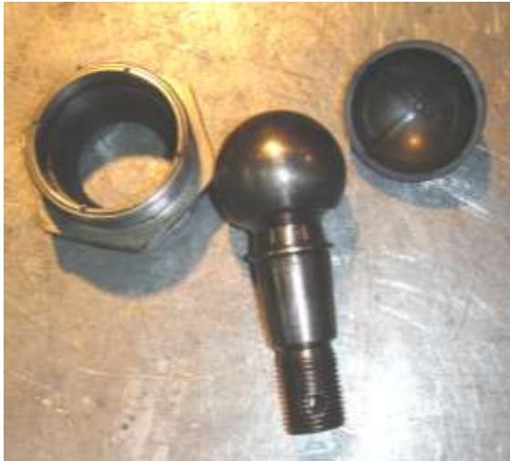
And this is the joint in pieces. The Shadow and Spirit used 'plastic' very slippery cones and cups seen here for the ball of the joint to turn in. With liberal greasing there is little friction and little wear.
