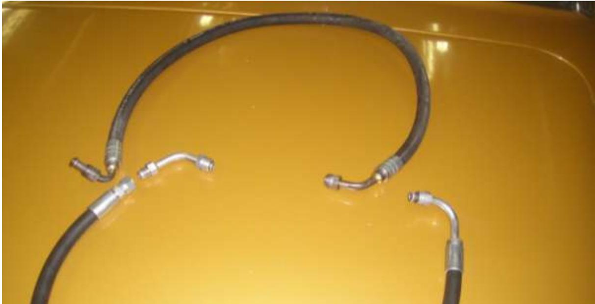
So here is the solution, the lower hose has been made up but the end into the box has been modified as an attachment. The latter is made up loose and the hose installed. The end nipples are nipped up, the hose support bracket fitted and last of all after assuring yourself that the hose is perfectly relaxed, the modified connection to the hose at the box end is tightened!
