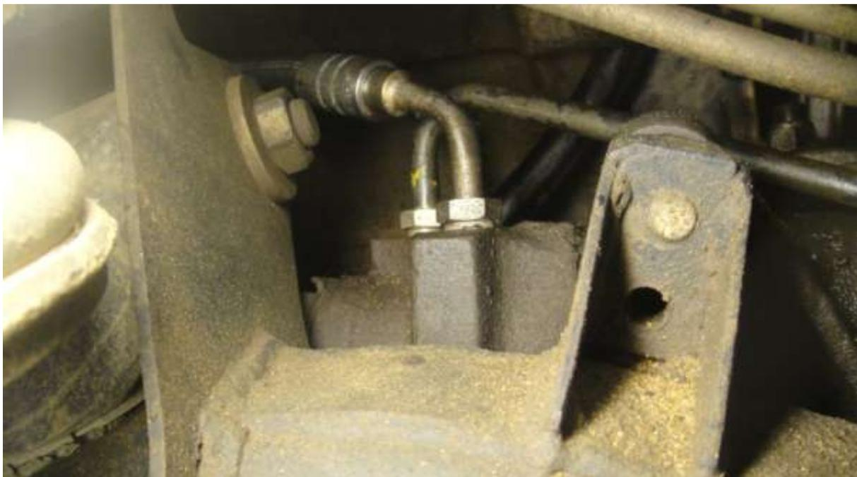
All Shadow I's (sic) still functioning will have had their high pressure hose from the back of the power steering pump to the top of the steering box replaced at some time. Some
