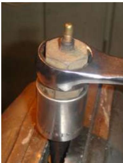
At left is one way of holding the switch while undoing it since the two pieces of the body are usually very tight. The socket is held by a short extension piece which is clamped in a vice.
