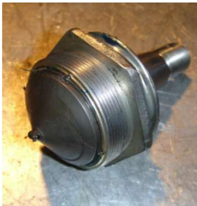
the lower and upper wishbones down to their limit and there was then a distinct hollow sound approximating to 'BOCK'. The noise was not unlike that of worn telescopic shock absorbers but I eliminated that diagnosis by their replacement soon after I got the car.
