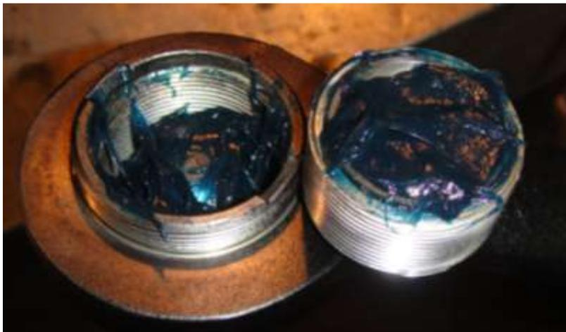
Here the bits have been refitted with lots of wheel bearing grease and the cap is ready to be screwed down and adjusted.
