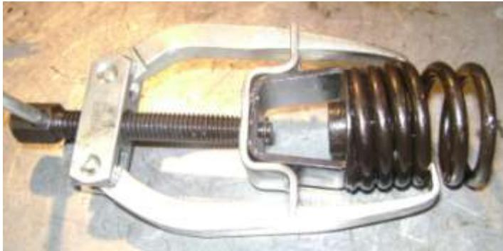
At left is the tool now used for removing valve springs. The legs that grip the coils are offset to allow for the coils and the cap is pushed down by an adjustable saddle seen here.
