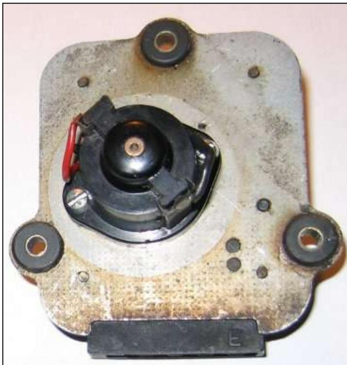
Here the motor cover has been removed exposing the little noise maker we are so familiar with. The tiny bronze bearing seen in the middle of the motor casing is an Oilite bush.
