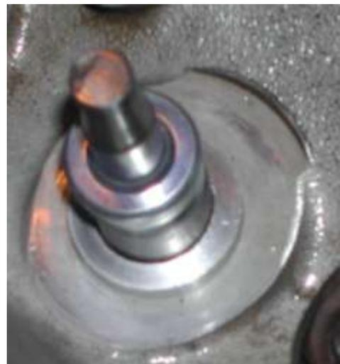
At right can be seen a locating ring that is placed over the guide which is made up to replace the original small 'top hat' since that item and its spring has no function with the new seal. The 'rim' of the discarded
