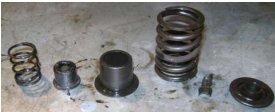
The bits above were removed from the valve in the first picture. The 'top hat' and smaller spring at the left, fit over the old seal and the top of the valve guide, these in turn are held down by the larger 'top hat' which also has the job of holding the bottom of the valve main spring in place. The last two items are the spring cap and the little collets that fit in the groove at the top of the stem which can be seen in the first picture.
