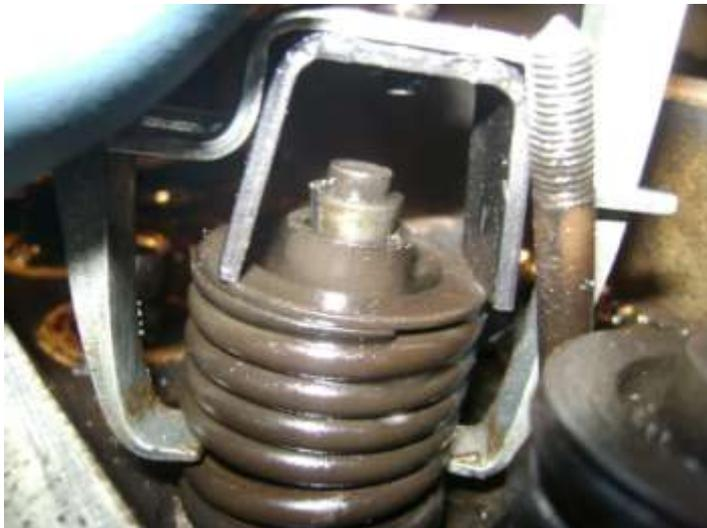
At left is a spring compressed and pushed down the valve stem to reveal the two collets waiting to be plucked to security
