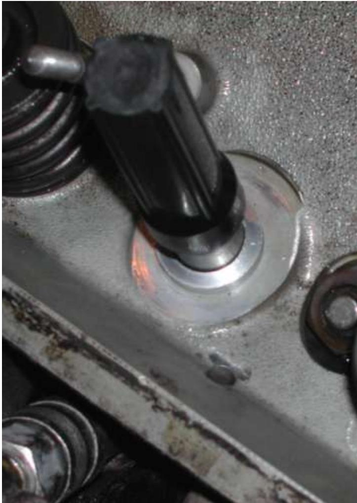
At left is the simple plastic tool to drive the new seal over the end of the valve guide. All that remains is to reinstall the main valve spring on its 'top hat', the retaining washer and the valve collets.
