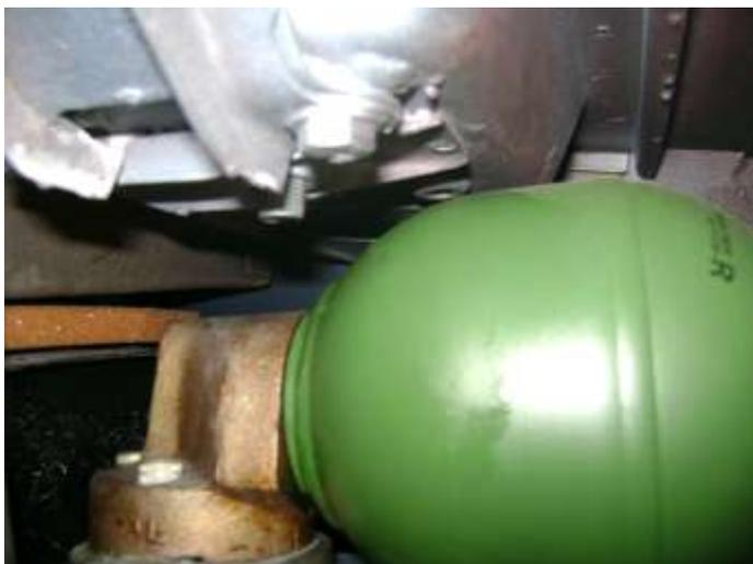
The top nut presents a different problem as it is under the adapter mounted on the top of the strut that carries the gas spring. These incidentally are often referred to as accumulators since they look the same albeit larger and they have the same construction. The adapter is recommended by the workshop manual for removal when replacing the spring for reasons I have yet to fathom! The thing is bolted to a plate
