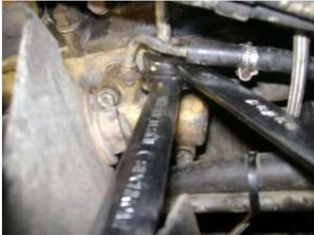
Since this accumulator had all its supporting bits it was safe to undo all the pipes and bolts and the assembly would just sit on the support brackets.
