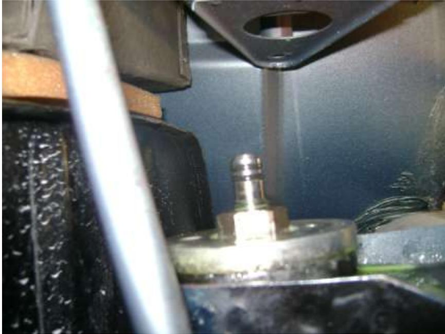
When you have managed to remove the mount and gas spring here is what you find, that is after you have climbed out of the boot (trunk) straightened your back and had a pick-me-up! Note the two 'O' rings on the top of the strut mount. It is important that these not be damaged. It is fairly easy to slice them so that when the whole lot is back together you find a nice little leak from under the
