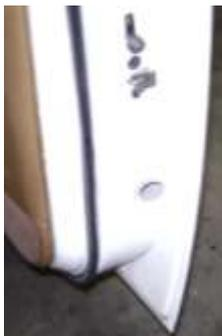
In the automotive world of survival, these little safety lights (this one has been removed for repairs) on the trailing edge of post55 cars would have to take the prize. The body of the light is rubber and the lens is glass, yet it stands slamming a zillion times and even the globe seldom fails. To change the globe very carefully prize the whole lamp out of the door bearing in mind that it is old rubber. If you stretch it unduly the lens will
