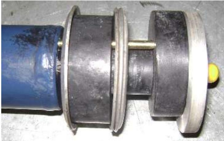
Here the bits are assembled to show their relationship. The large gap is where the assembly passes through the body. The upper rubbers have apparently been modified since the section surrounding the distance piece has been considerably beefed up over that used in early cars.
