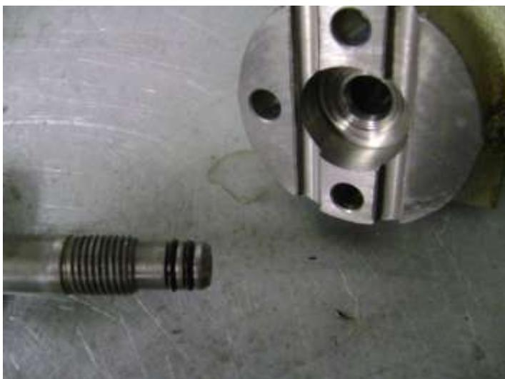
The workshop manual for some reason recommends removal of the gas spring mount seen in the picture when changing the gas springs. This is not only unnecessary as the gas springs (which in appearance are similar to the main hydraulic accumulators) can be screwed out of the mounts in situ. Apart from the awkwardness of removing the mount there is the inherent danger of damaging the 'O' rings seen here at the top of the strut. If they leak they will rot all the top strut mounts.
