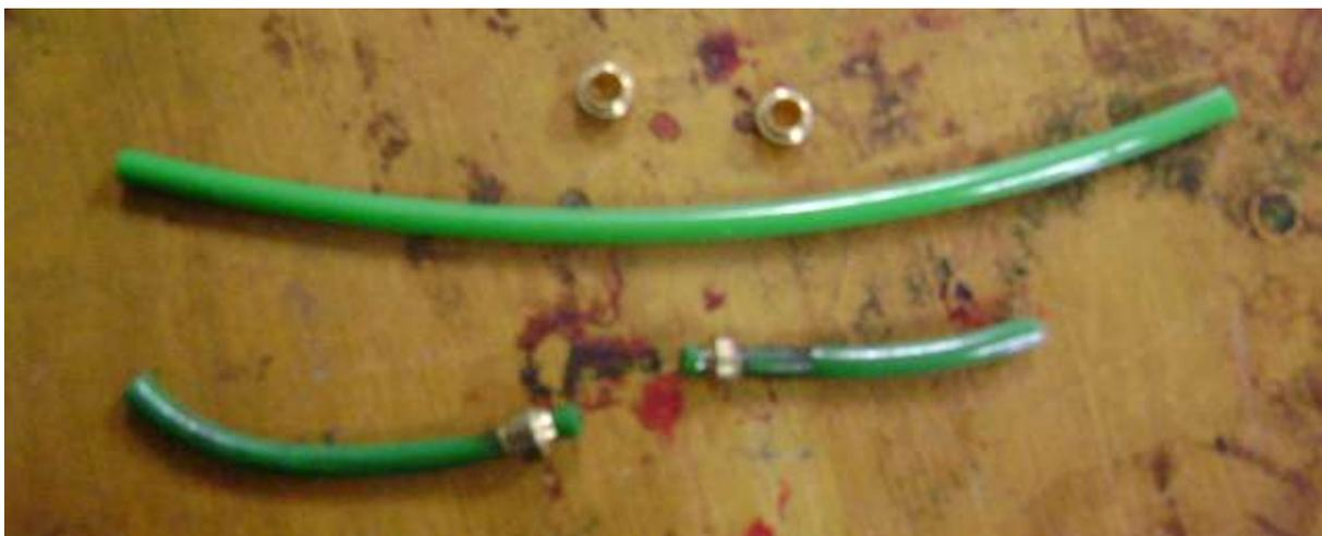
The last minor detail to mention in all these words is the little tube from the strut to the body seen in the first picture. Given the work the internals have to do in these struts some fluid (LHM) gets by the various seals. Rather than have them dribbling all over your nice terrazzo driveway, the stuff finds its way back to the reservoir via these little tubes. Since the whole strut is continuously wobbling it is well to keep an eye on these and renew them if they leak!
