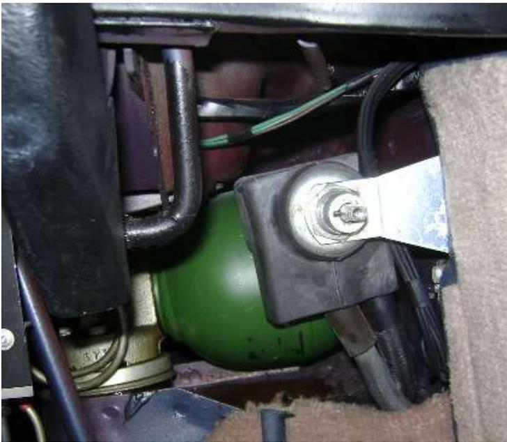
The only difficulty with this job is the nuisance of having to remove the battery master switch on the right hand side of the boot to get at the gas spring behind it. Before attempting this you will of course completely disconnect the battery won't you!
