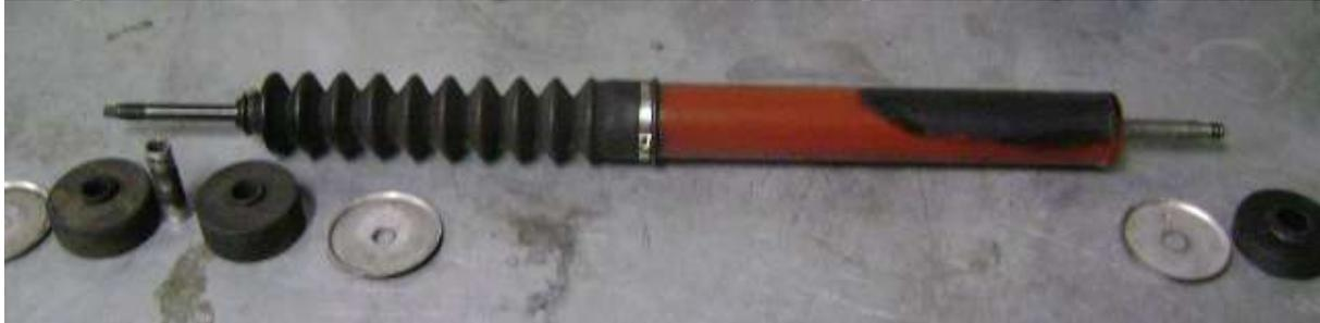
Here is the strut removed and stretched out. Unlike shock absorbers these can be emptied of fluid simply by pushing the plunger up the barrel. Be very careful to assemble the rubber bushes spacers and separation washers in the correct order which is shown clearly in the workshop manual.
