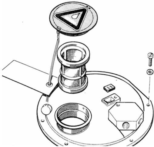
Initially, SZ cars' reservoirs were a simple affair as seen at left. To top up the cap was simply prised off and the fluid poured in. Note the label and warning logo on the cap.
