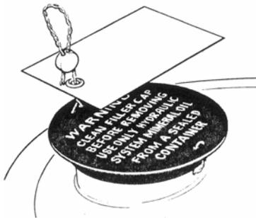
To try and avoid these accidents, the Factory commenced wiring the caps in place and locked them with lead seals. Multi lingual labels were conspicuously mounted but still contamination occurred.
