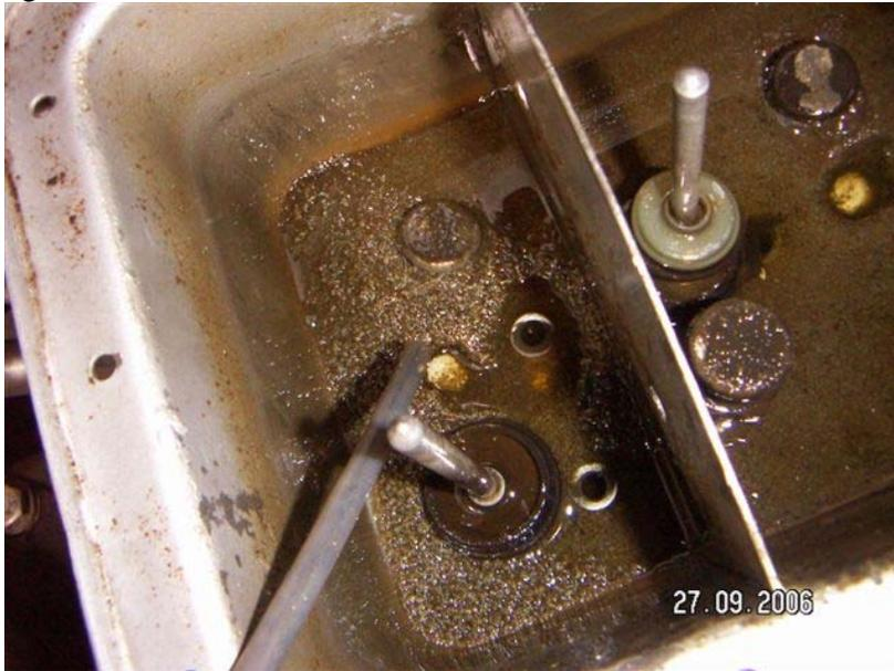
Next step was to carefully unscrew the accumulator charging screw caps which on a Shadow I you can do, unlike its immediate successor.
