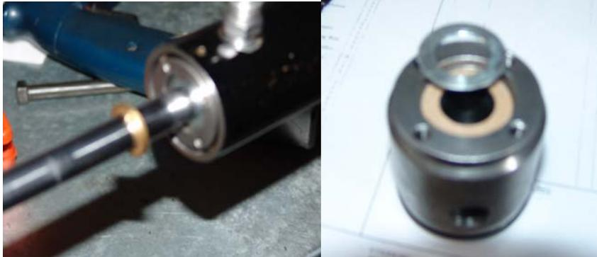
Re-assembly is straight forward. The Factory make a up a kit for the operation which includes all the seals and a new retaining circlip for the piston (not pictured).
