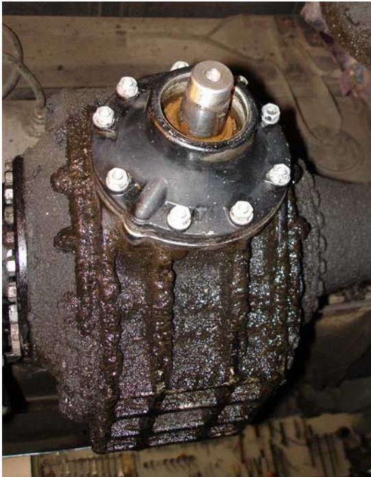
The flange removed – note the keyways. The bulge at seven o'clock is a return duct to carry oil away from the seal that has worked its way through the pinion bearing.
