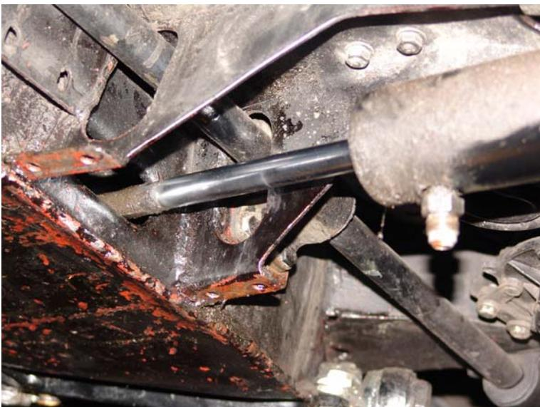
The plunger emerging from the rear of the power cylinder and passing through the front cross member. Here the lower support plate has been removed and the cylinder pulled well forward. The front anti-roll bar can be seen above the plunger.
