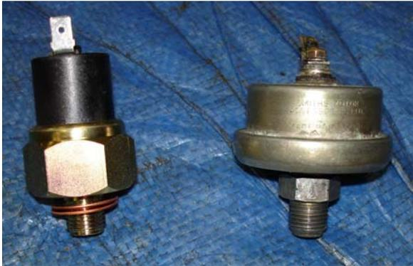
One of the original senders seen on the right in the picture here with a modern type beside it. The older sender had a requirement to be fitted by selective choice of washers so that the gauge was in a particular position. This is apparently not a requirement of the new unit.
