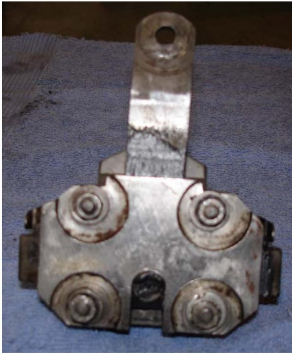
the combined hydraulic double acting piston that applies the rear brake shoes in your Cloud. If they should fail the wide rod seen protruding from the assembly, working through rollers and cams manually applies the same brake shoes.
