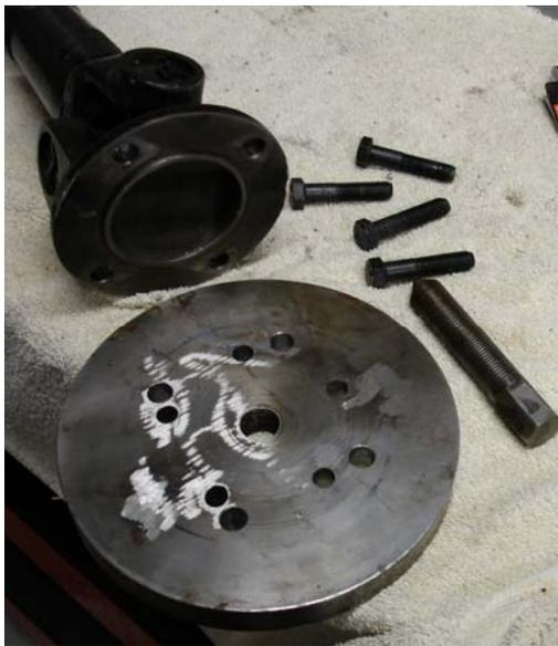
Do NOT use a leg puller or you will most certainly bend the flange and even run the risk of breaking it! Go to your local friendly fitter and turner and ask him to make up a stout disc of good steel about an inch thick with a central threaded hole. He will tell you where you can get a suitable mandrel (the high tensile pointed bolt screwed through the middle).
