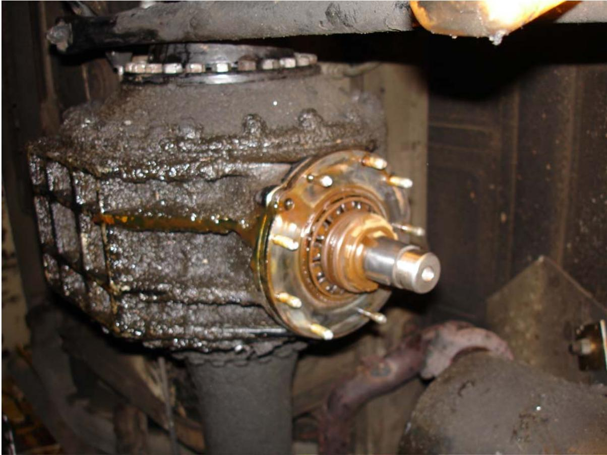
The seal carrier is off. The oil return hole can be seen along with a conventional scroll to encourage oil to go home.
