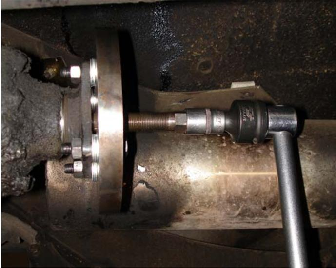
You should also go to your nearest bolt shop with one of the propeller shaft flange bolts in your greasy hand and purchase four high tensile bolts and nuts, the same diameter as the flange bolts but long enough to go through your puller and the flange leaving enough to get the whole new nut on.
