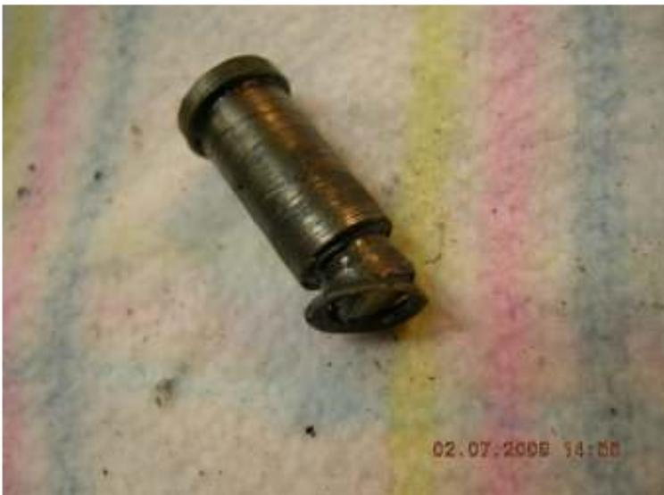
**Worn & broken cam retaining pin**
