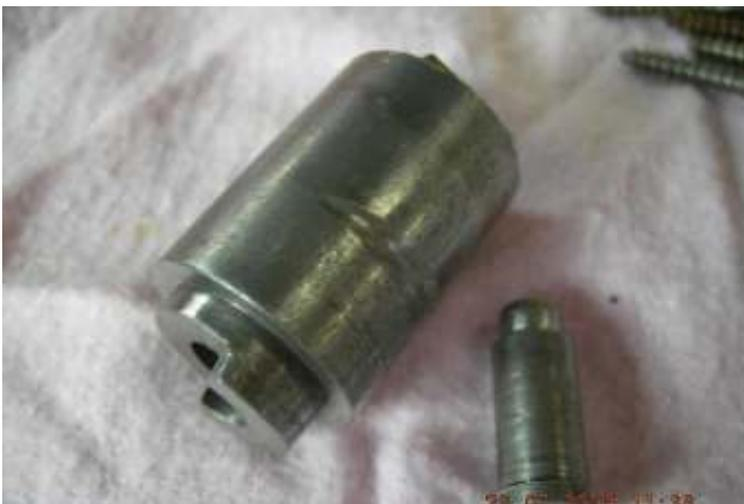
**Worn CAM with broken pin**
