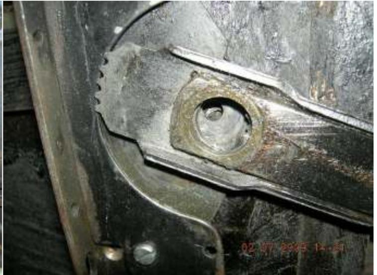
**Worn regulator with missing cam**
