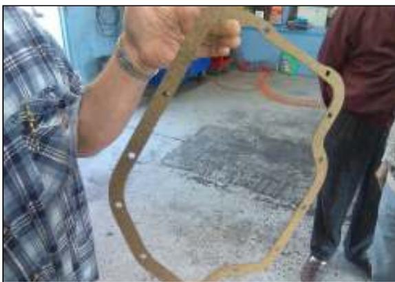
**The pan gasket and replacement filter for the Turbo 400 transmission is pretty much a 'bog standard' GM part and can be obtained from any transmission specialist**
