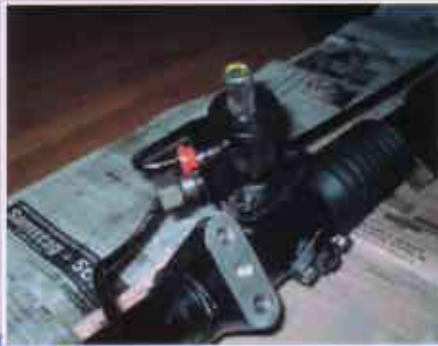
Above: The late-type rack, showing the cast mounts integral with the aluminium and housings and the external backlash adjuster. Early types have their mounts fabricated and welded to the end-housings.
