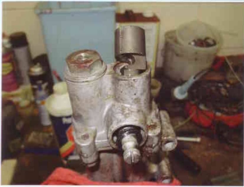
Figure 2 Removal of piston.
