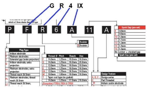
As an example, the NGK GR4IX spark plug is now the only plug to use on all SY and SZ cars until Model Year 1994. The gap is 1.0mm (0.040").
