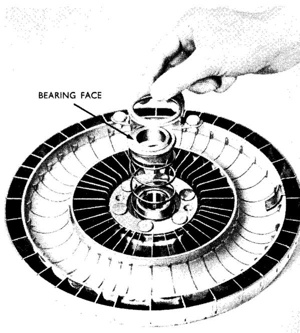
**Fig. 4. Removing torus relief valve**
