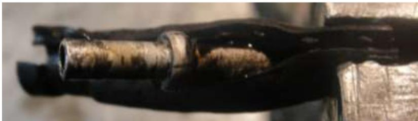
The restrictor being prised surgically out of the old bit of tubing.
