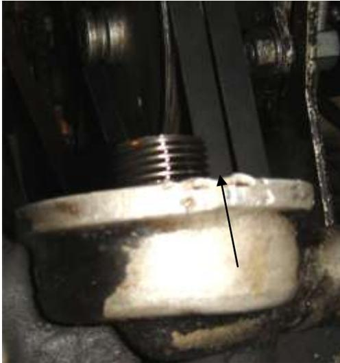
At left is the mounting face of the engine oil filter on a low mileage Turbo Bentley. Some very lazy person who either did not have a filter wrench or couldn't be bothered getting one apparently used a cold chisel! This explained the little dribble of oil at the front and possibly the higher oil consumption.
