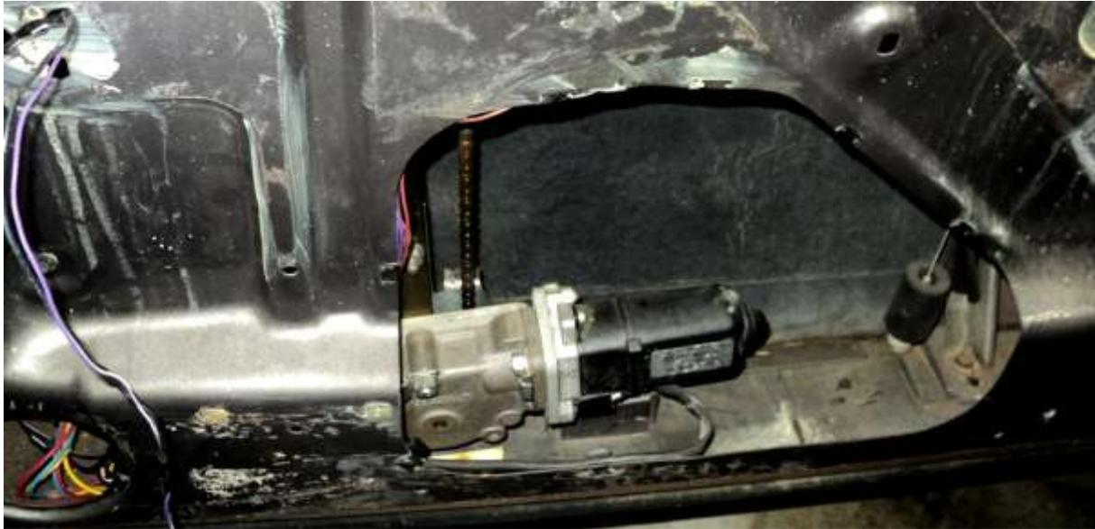
Well the door lining is off and there is the motor which is held onto the winding gearbox by just two studs and nuts. At lower left the broken coupler is emerging from the gearbox with the aid of your dentist's probe. Below that is a better view of the motor shaft adapter with a cross pin that engages the coupler and if you climb inside the door you can see a similar adapter on the input shaft of the gearbox.
