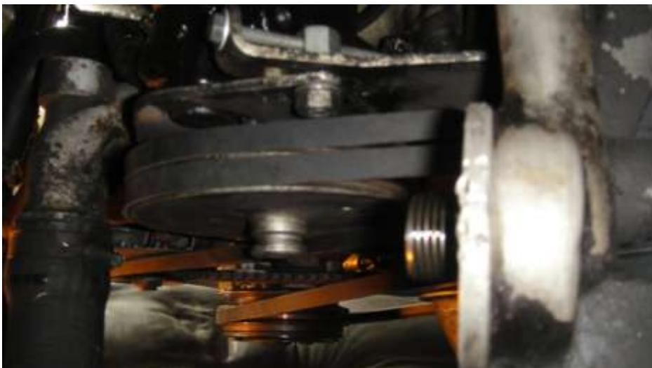
And here is the tensioner for the power steering pump, accessed from below.
