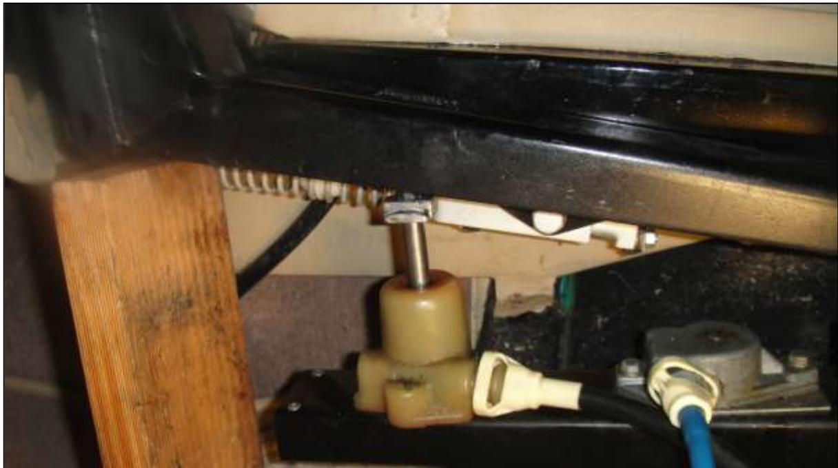
The blue flexible cable, one of two, drives the gearbox that traverses the seat fore and aft.
