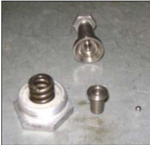
This is 'all' there is to these joints. The tapered pin at the top rides on the little ball bearing which in turn sits in the cup between them. The spring allows the joint to flex when the suspension moves to extreme positions.
