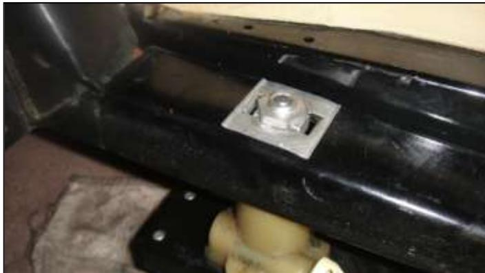
At left is the mount for the top of the jack. The screw shaft is very firmly anchored in the two securing plates to prevent its turning during jacking. The seat here is at maximum height.
