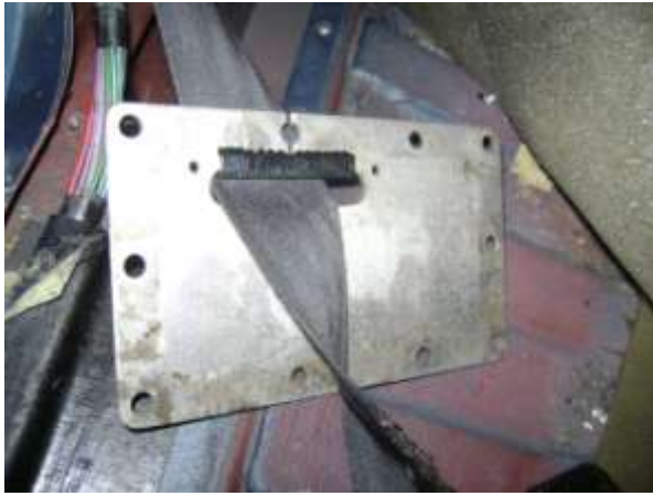
Here is the plate showing the insertion slot and the simple remedy to prevent chaffing of the webbing.
