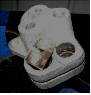
At left is an over-flashed picture of the pivot pin having been pressed out of the back of the wheel cylinder. This took some tons to move after much soaking in WD40 and applications of heat! The crud in the hole can be seen clearly.
