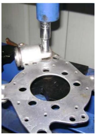
enough to overcome some friction in the shake back stops moving the shoes and pushing the wheel cylinder pistons back slightly so that the shoes finish up very lightly touching the drums. The next brake application repeats the process but the shoes have merely thousandths of an inch to travel to do their job!
