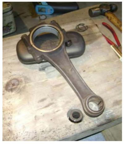
And here is a very special tool. The requirement was to support the piston while the gudgeon pin was pushed/pressed/bashed out without distorting the piston! Complicated cradles were planned but a solid pine block with a large hole bored through it did the job. Here the piston has been removed and the gudgeon pin waiting to be collected. I noted that the etching on the end of the pin was always facing the same side as the etching on the end of the connecting rod!
