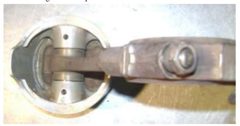
gudgeon pin is retained in the piston by expanding circlips.
