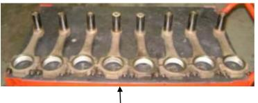
And here they are all lined up like kids for their daily mouthful of Saunders Malt Extract (remember?). These rods have a frightening task just staying in one piece so they are made, balanced and inspected with great care. The bolts are equally critical and if there is the slightest doubt about one it must be replaced. The carnage that follows the breakage of one of these little bits is heart rending!
