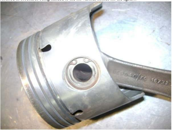
Here we have the piston nice and clean showing its circlip ready for removal. One of the nice touches in manufacture is that the piston is stamped with its bore number and grade, the gudgeon pin has the bore number on it and the connecting rod AND cap have the bore number on them!
