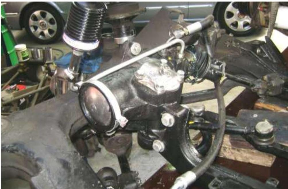
The steering box is left attached to the sub frame. The front cross member is actually bolted to the box and carries most of the weight of the engine. The high pressure hose that supplies pressure to the box can also be seen.
