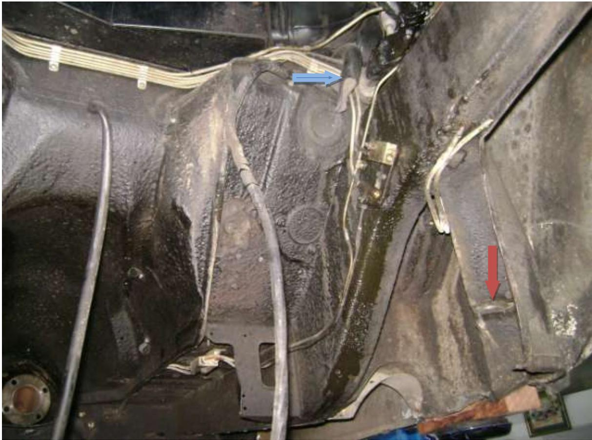
This is a good time to tart up the parts you can never really get to. The left rear sub frame mounting point (arrowed red) can be seen together with provision in the toe board for left hand drive cars as well as the rat trap mount which also changes side across the Atlantic. The blue arrow points to an often obscenely described rubber pendulous, moulding. There are two of these which drain the heater box, the top of which is open to the weather. The end of
