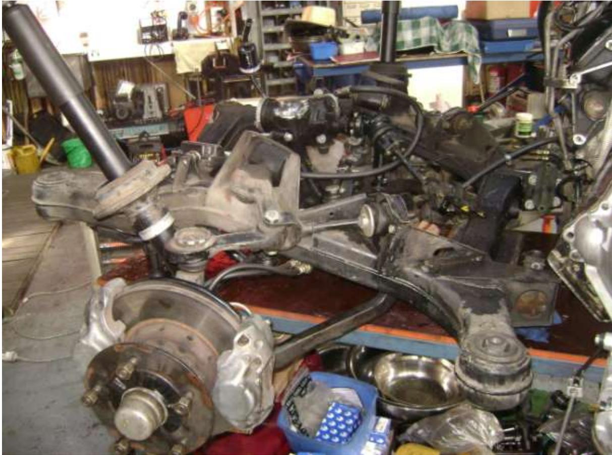
What a mess but after your eyes have focussed you can see most of the sub-frame, the shock absorbers, the steering box on the far side, the steering shaft and CV joint. The mounts on each corner can be seen also. These are the rubber silentbloc type and eventually perish. A
