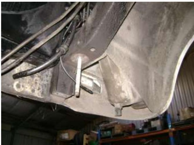
At left is the right front mount for the sub frame still with its bolt hanging through. The angled pipes are on their way to the bottom of the radiator core with the transmission fluid and the angled box tucked in behind the mudguard is the bottom end of the air cleaner! The bit hanging off the latter's bottom is a water drain should you do some river fording.
