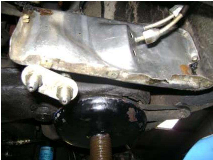
The aluminium plate at the left is the front closure for the rattrap. The pipe ends at left are the two flexible lines between the body and the sub frame. Until early in the Spirit run which is basically the same it was thought provision should be made for movement between the two. Later Sprits have simple rigid pipe connections. These lines carry hydraulic fluid from the brake distribution lines to the
