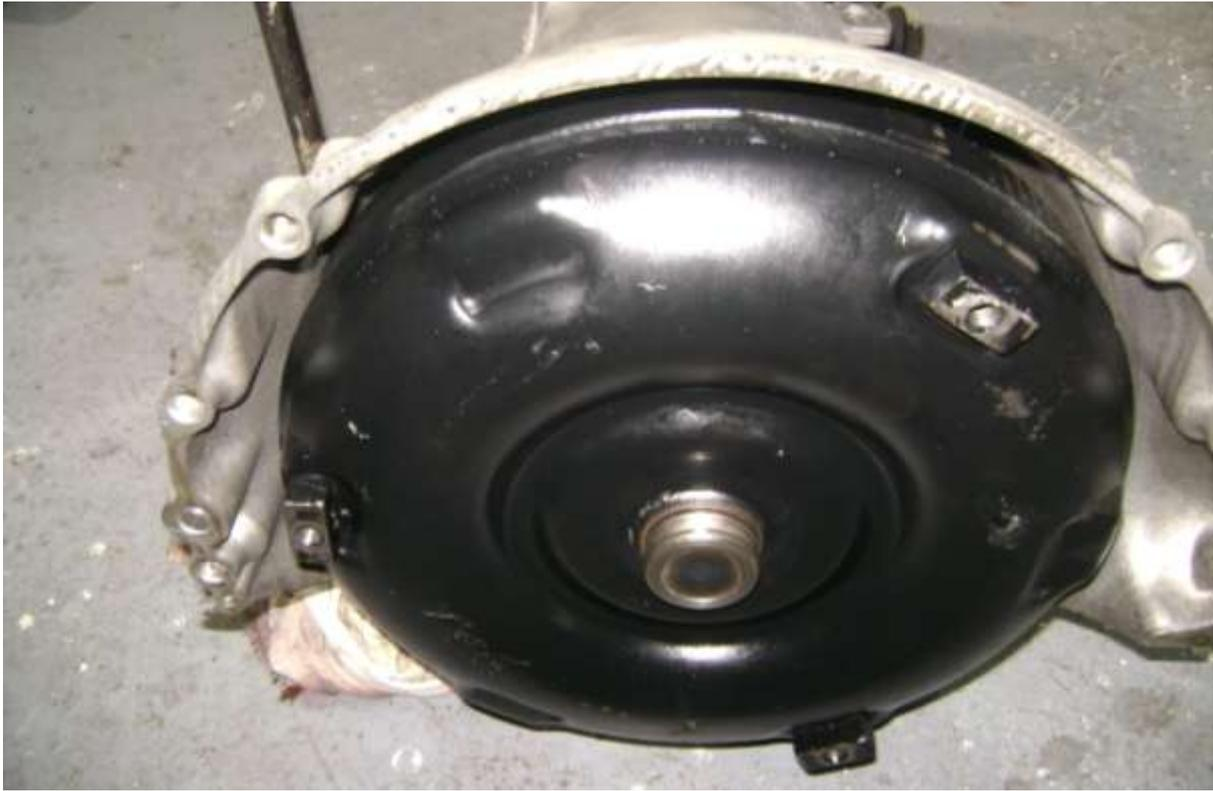
The front end of the converter showing the three mounting points. The converter is bolted on through the drive plate, the bolts accessed through a small plate on the underside of the main housing. Converters are common to many cars. If a transmission is overhauled and there is the slightest trace of damage in the sediment the unit is sent to specialists to be cut open (they are a sealed unit) cleaned out overhauled and returned as good as new for a very reasonable fee.
