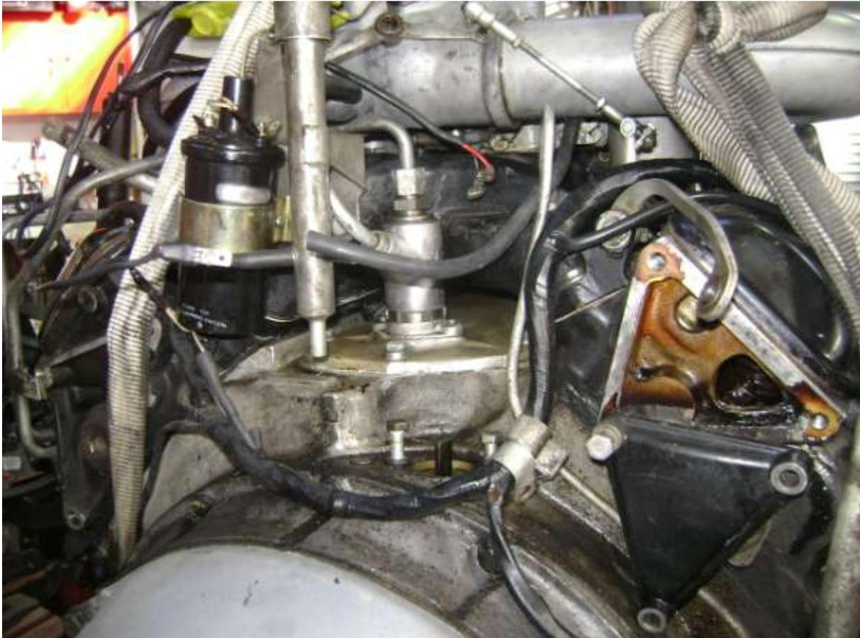
Have you ever wondered what all the mess is at the back of these engines – well here it is. Wiring looms, some of which are seen here plug into points on the engine toe board. They are unhooked from around the engine compartment and simply left on the top of the engine when it is removed. The hydraulic pump for the number two system can be seen attached to the engine valley plate. The cylindrical gadget to the pump's rear is the collector of noxious overflows etc from the fuel system.
