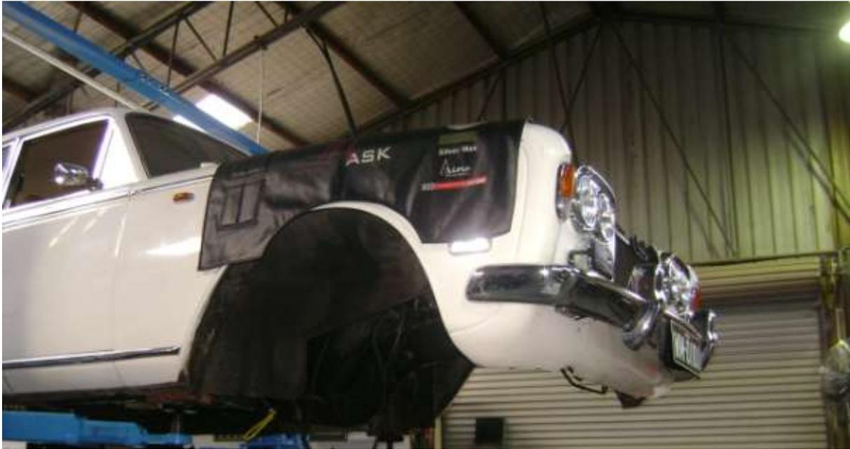
Surely this is a testimony to structural engineering. Even with the engine and transmission in place the lifting points are the same – there is no sagging!
