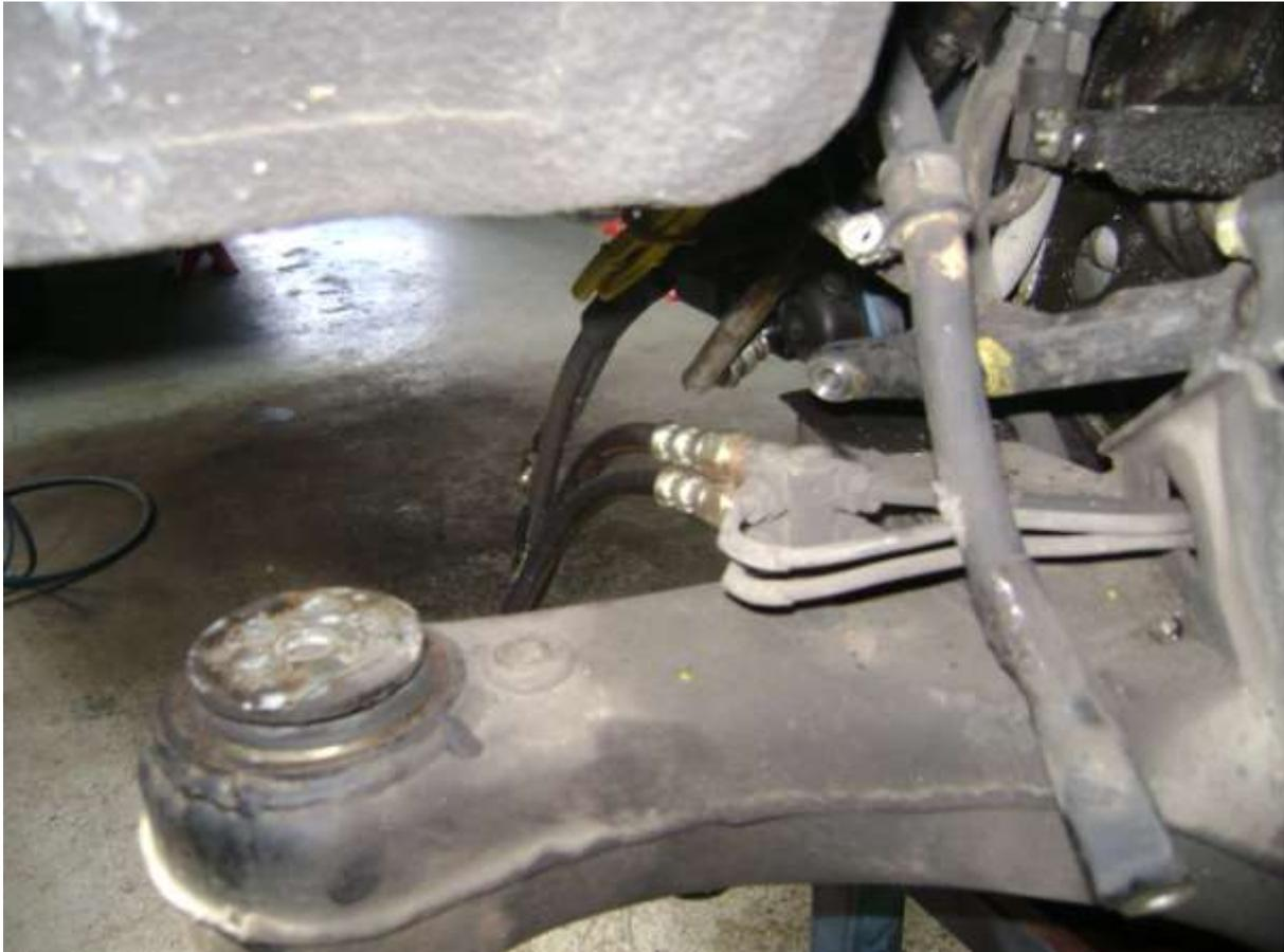
The connecting hoses seen on the previous page can be seen dangling from the junction blocks mounted on the rear of the sub frame. One of the four mounts of the frame to the body of the car is seen at left. The heavy cable draped over the frame brings all power to the car from the rear mounted battery and connects directly to the main starter terminal.
