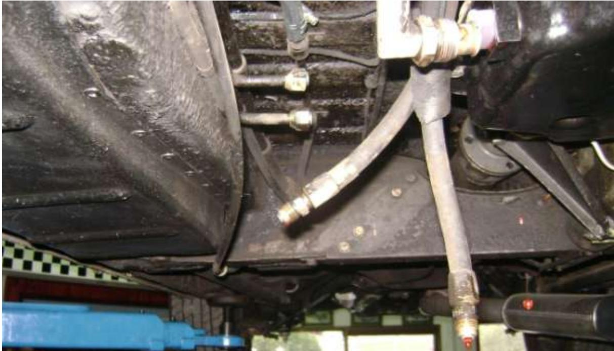
These two flexible lines send and receive transmission fluid via steel pipes seen to their left close to the car floor, to the lower end of the radiator where a separate core is fitted for cooling. The output flange at the rear of the transmission can be seen unbolted. It is not necessary to remove the propeller shaft. The cover for the legendary rat trap is at left.
