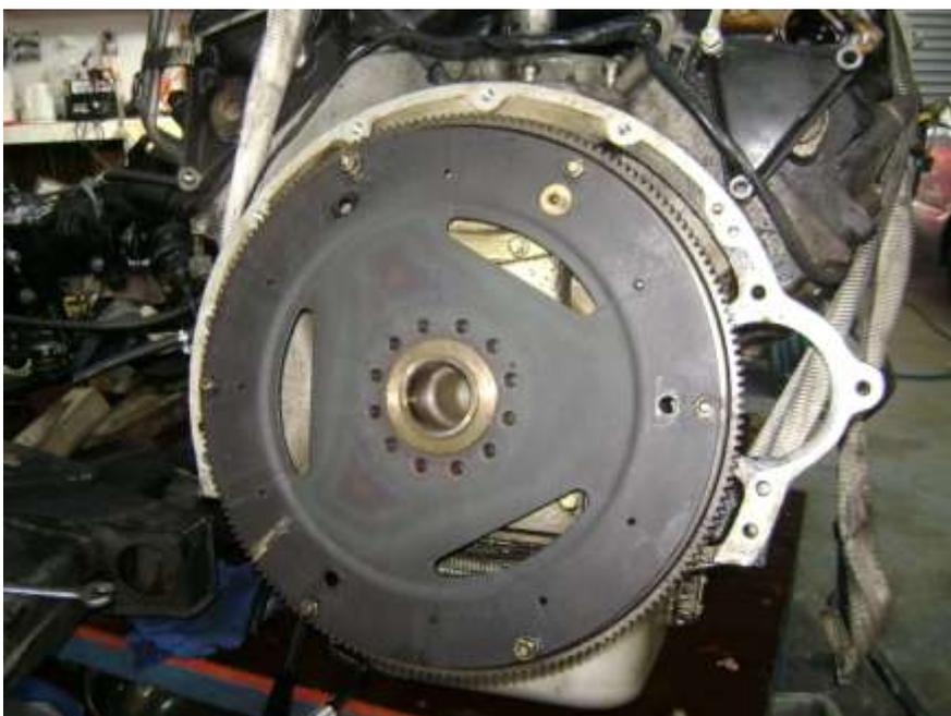
The transmission has been removed. Generally cars with automatic transmissions do not have flywheels since the torque converter when bolted to the drive plate seen here is sufficient in mass to perform the function of the flywheel. The converter is help on by only three bolts the holes for which can be seen here. Later cars used four bolts.
