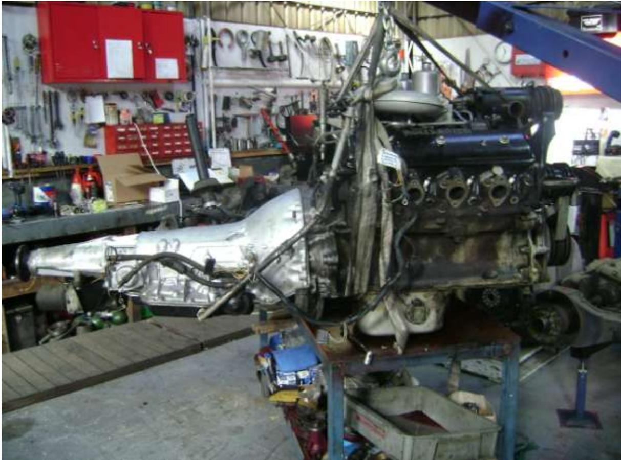
Above, the engine and transmission have been separated from the sub frame. The extraordinary route the transmission filler pipe takes can be seen clearly. Note the slicks on the side of the engine block under the exhaust manifolds indicating the usual tell-tale weep holes leaking.
