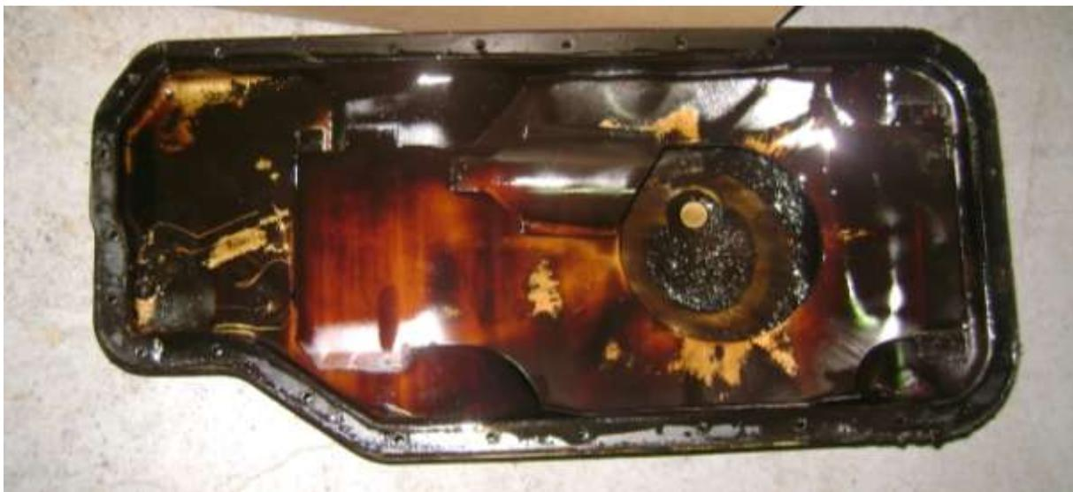
The sump. They are not easy to get off but well worth the effort. It is likely that this engine at some time was sufficiently overheated to destroy some of the tension in the piston rings resulting in 'blow by' of gasses which contribute to the mess seen above. The sediment can get to the point of restricting the intake filter for the oil pump.
