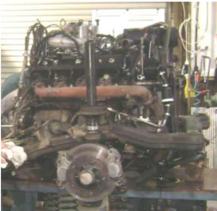
The complete mess has been left sitting on a very stout steel table and the body lifted away. The front mounting points for the sub-frame can also be seen as well as the anti-roll bar mounted beneath.
