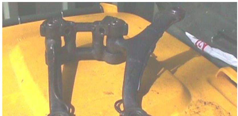
The central steering relay levers of John Beagle's R Type
