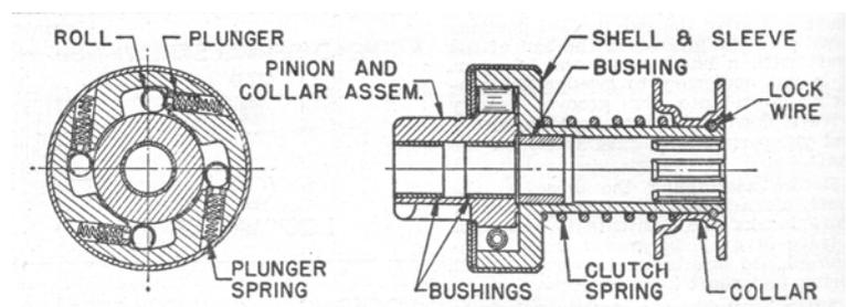
From the Silver Cloud II series on, multiple disc clutches were dispensed with in favour of the over running clutch above. These can be overhauled by a specialist firm in Melbourne. They should be tested for slipping at 25 – 30 ft lbs with a tension wrench
