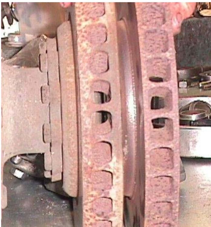
An appalling piece of maintenance. The brake rotor on the right has been ground way beyond the minimum permitted. The rotor on the left is of original dimension
