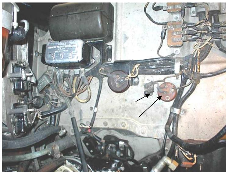
As fitted to the first V8's. The Otter switch is on the left
