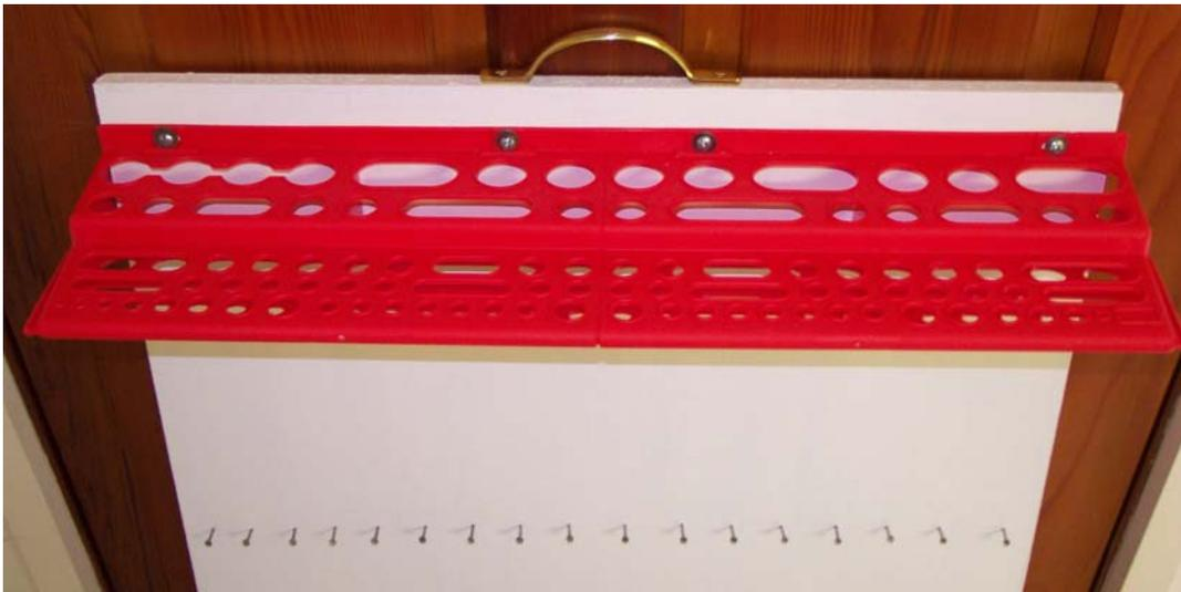
This photo shows the essentials. A piece of 18 millimeter chip board with a tool rack near (but not at) the top, a row of nails below this and a handle on top.
