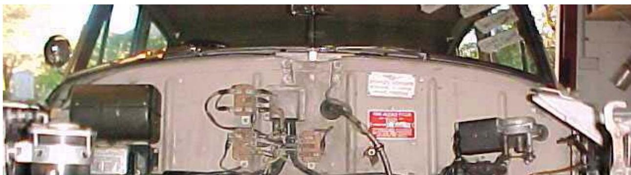
**The flasher relays for the fog lights fitted to an S2. The flasher units are located above the steering column behind the dash panel**
