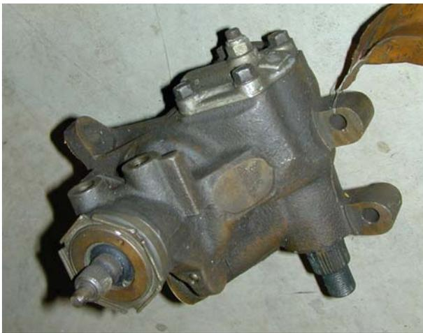
The Saginaw manufactured steering box fitted to Shadow I's (sic). The main adjusting point can be seen on the top with its locknut. The large nut to the front is for setting the pre-load on the input shaft. It is very unlikely that you will need to fiddle with the latter
