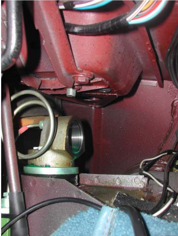
And here is the mounting block on top of the right hand strut showing the threaded entrance for the gas spring
