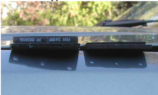
Another reminder to keep brake pads in mind. Seen here new on left worn to the limit on the right.
