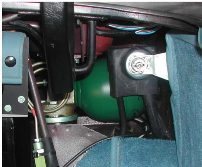
And here is what you will find having got the back of the boot uncovered. This is the right hand side showing the sphere and in front of it the battery switch which clearly needs to be moved to one side. The Factory recommends that the mounting block for the sphere (seen behind the coiled pipe) be removed to unscrew the sphere. . This is unnecessary as there is sufficient room to get the thing out without trauma. The left hand side is very accessible
