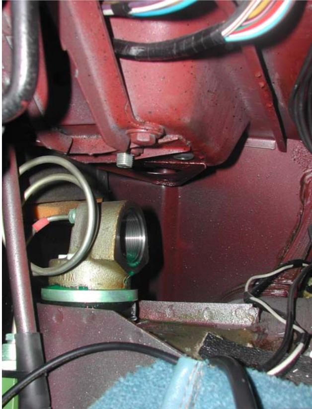
And here is the mounting block on top of the right hand strut showing the threaded entrance for the gas spring
