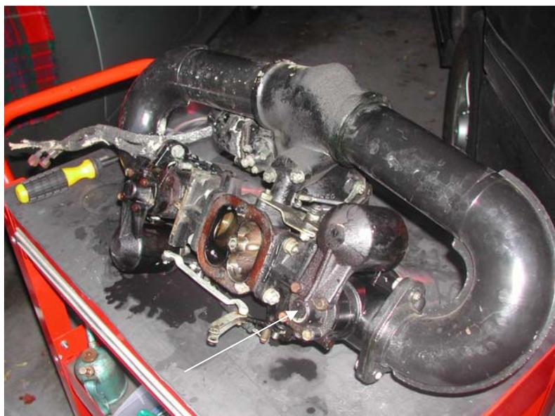
Replacement of the diaphragm on the larger engines is not major thanks to a simple fixing method of the induction system. The above picture is of a Cloud III which sprang a leak. Between the two carburettors there is a very long bolt that goes down into the engine. Having undone some pipes and the odd wire, this bolt can be removed and the entire induction system removed.
