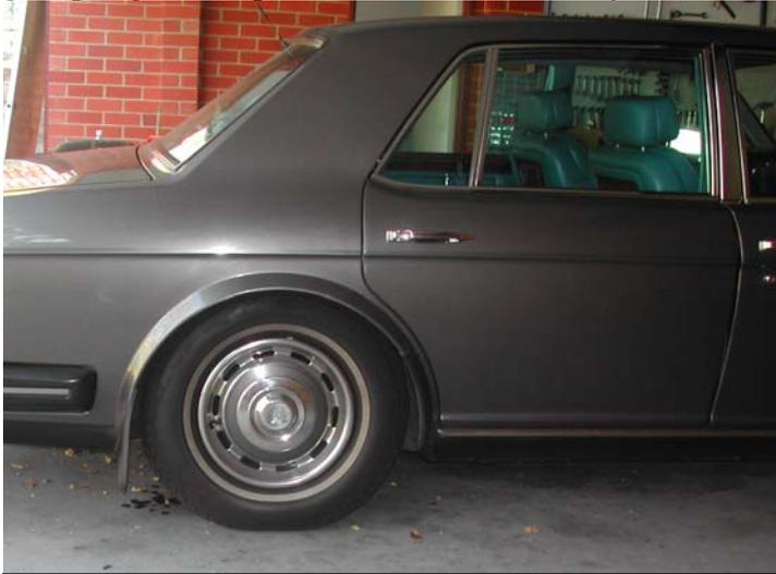
Sitting on its haunches having had its struts exhausted. Taken springs that are holding this car up are there to avoid the Citroën malady of the car collapsing when the suspension fails.
