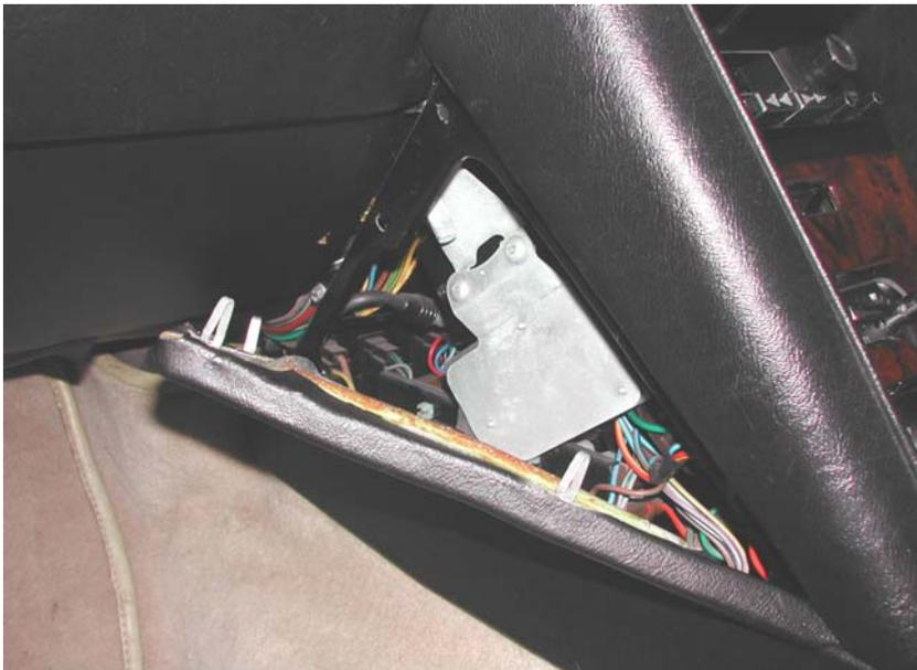
Everybody knows how to get into the central console don't they – but for those that don't here we are – same clips as used on the Cloud door panels. Use a wide blunt knife to lever the panel out of either side of the console. You will need this access to replace the globes behind the heater switches. What globes? Those expensive tiny 14V bulbs with blue caps over them – have a look and see.
