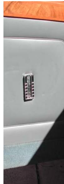
On post-war cars the panels are held on the door by patented clips similar to those used in most cars. Beware with later cars particularly the Spirits and Spurs that there are also hidden screws usually embedded in carpet.
