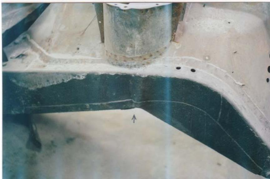
Nick Lang sent this interesting sight of the left hand forward member of a Shadow that had had a clout on the nose. Note the arrowed crinkle in the archway. Some of these car have had appalling frontals in their time and been very badly repaired. One quickly found clue to this is the absence of buckles or dents in the horizontal fillets either side of the radiator core also note the clearances between the leading edge of the tyre and the opening in the mudguard. They should be equal both sides.
