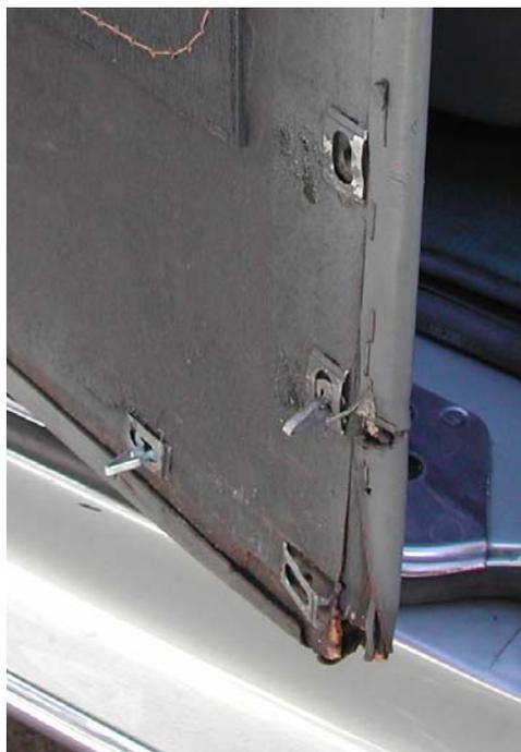
A fairly typical scene. Note that the leather has rotted away on the corner, a direct result of the bottom drain hole being blocked and the rain dribbling out of a seam at the corner. Also note the propensity of the panel clip holders to lose their clips or pull the holders out of the wood
