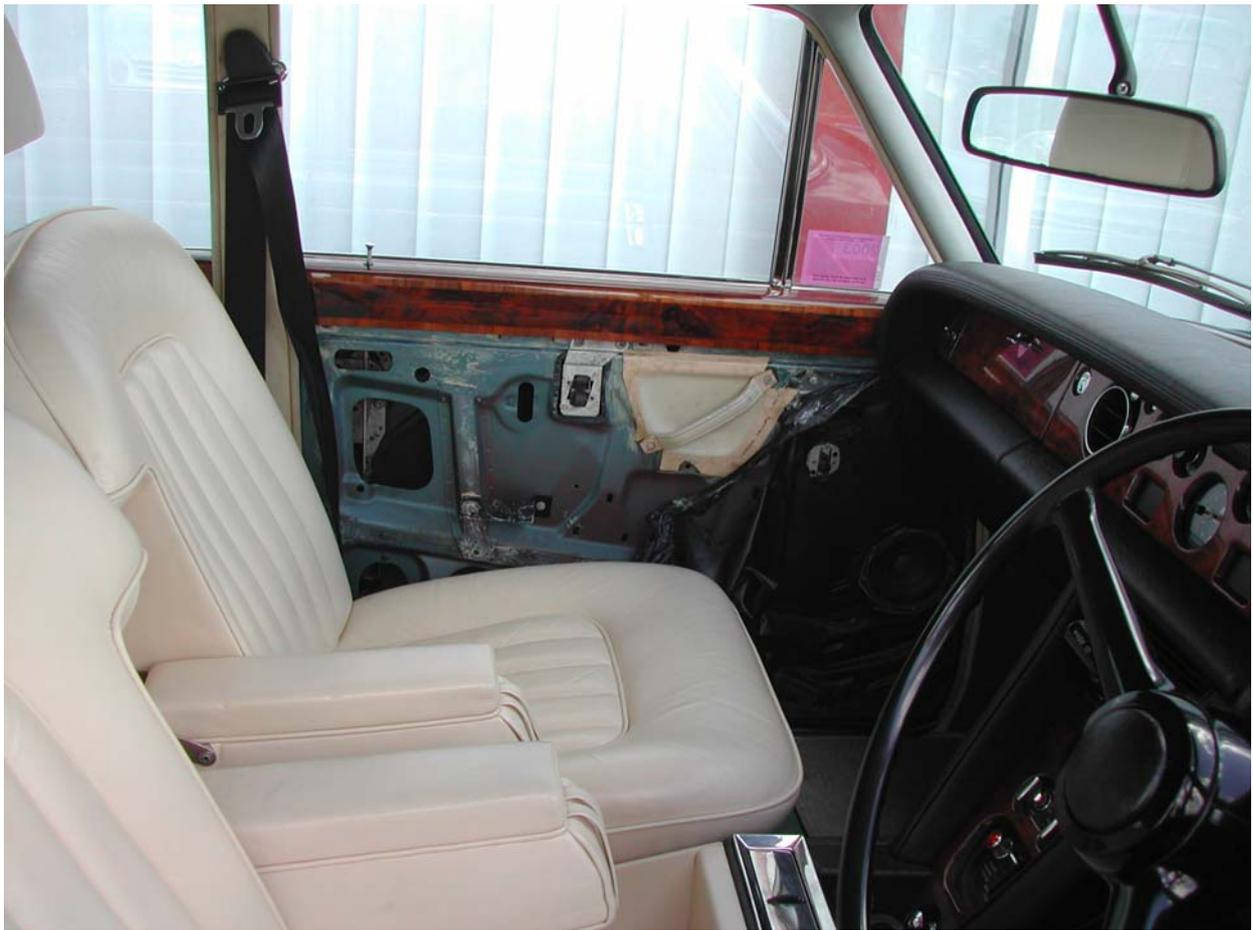
Seen at the recent Self Help Day organised at Neville's transmission place in Bankstown. Clearly an enthusiast ripping off the door linings to see what is going on inside, clearing out any muck neutralising any rust and lubricating the window mechanisms. Remember when replacing the panels to seal the door first with builders plastic and a non-hardening glue. This stops the moisture that gets into the door from rotting the timbers.
