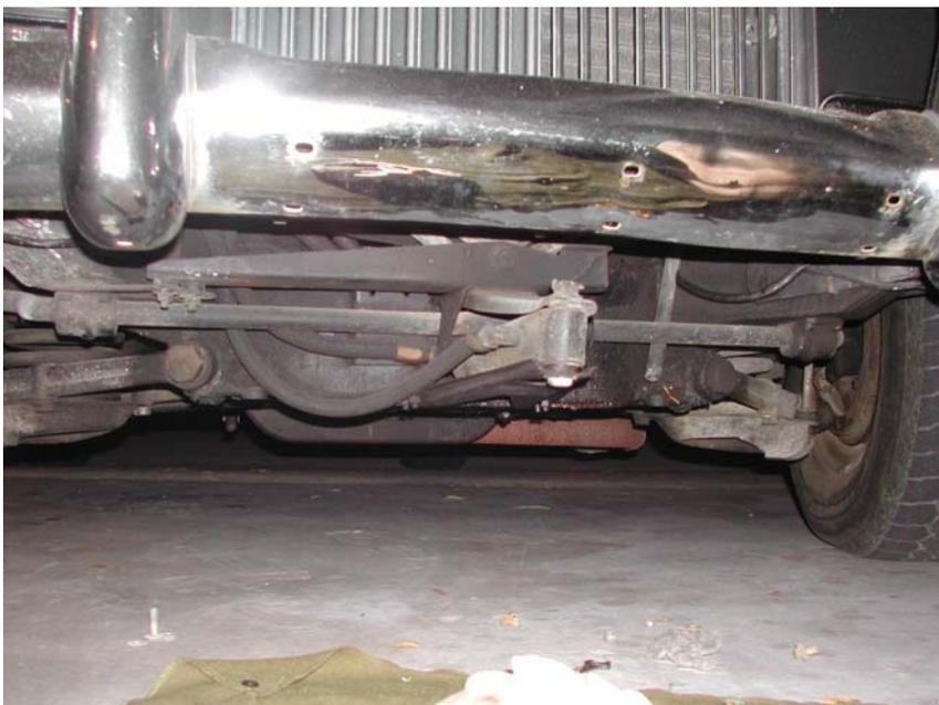
the steering box it was mounted ahead of the front 'axle' as a power ram which pushed and pulled the larger of the central relay levers. Of necessity the ram had to be low down and from the picture we all realise the consequences of ramming the thing into a solid curb!! The chassis on these cars, the last model to use a through frame was almost fragile compared with its predecessors. It was fabricated from heavy panel steel, immensely strong for resisting torsion and sagging
