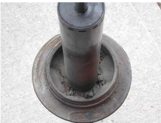
Typical accumulation of gunk - in this case some tar covered sticky gravel. All holes were blocked
