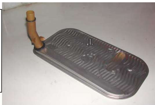
I am remiss in that Warwick Grigg sent me some pictures of his transmission filter and associated pick up tube. This is not them but a typical unit from all the Turbo 400 Transmission cars. As I recall Warwick pointed out that before you pull the transmission sump out of your car you should be aware that there are three 'O' rings required – all different sizes! Two are obvious here being at each end of the pickup tube, the other squeezes into the outlet/inlet used by the filler tube that goes into the right hand side of the sump.
