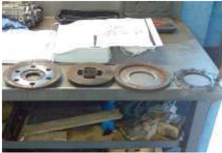
The Slipper Unit (Harmonic Balancer) Frequently Gets Clogged Up With Oil Sediment
