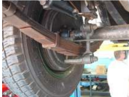
The Pad Here Is Under The Leaf Spring
