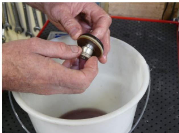
Another problem was that the reversing lights weren't operating and as both lights weren't illuminating, the first place to check was the fuse box. No blown fuses, so we checked the reversing light switch which is attached to the base of the steering column. There are two separate switches located near the steering box. One is for the reverse lamp, the other for neutral. They are operated by the same flap on the gear selector rod.
