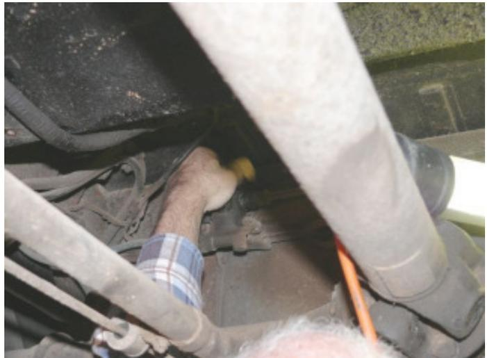
Removing The Main Fuel Filter Adjacent To The Fuel Tank For Cleaning. The Fuel Lines Were Also Cleaned.
